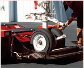
Raise the hydraulic cradle and you're ready to safely maneuver your plane into even the tightest spaces. To release the aircraft, lower the hydraulic cradle, detach the winch strap, remove the safety gate and back away from the plane.
