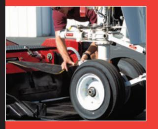
Drive up to the aircraft. Position the patented universal cradle at the plane's front wheel. Attach the winch strap around the plane's nose gear strut.
