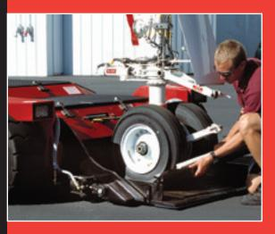
LEKTRO's built-in winch gently pulls the aircraft into the cradle — no heavy towbars or complicated attachments. When the front wheels are safely winched onto the cradle, simply insert the safety gate.
