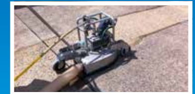
Small inaccessible areas can be handled with the hand cleaner MCD 360.
