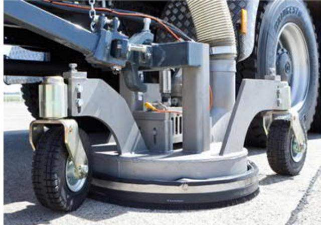
Retexturing and de-rubberizing „jetting devices“ (1 000 mm and 360 mm)
