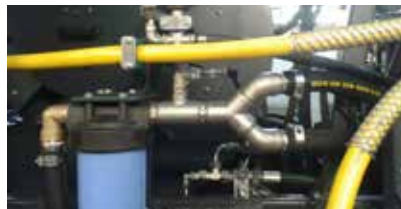
One of our features are the efficient and clean installation of the booster line (stainless steel) with a huge, final water filter and a filter inlay of 1 or 0.45 micron
