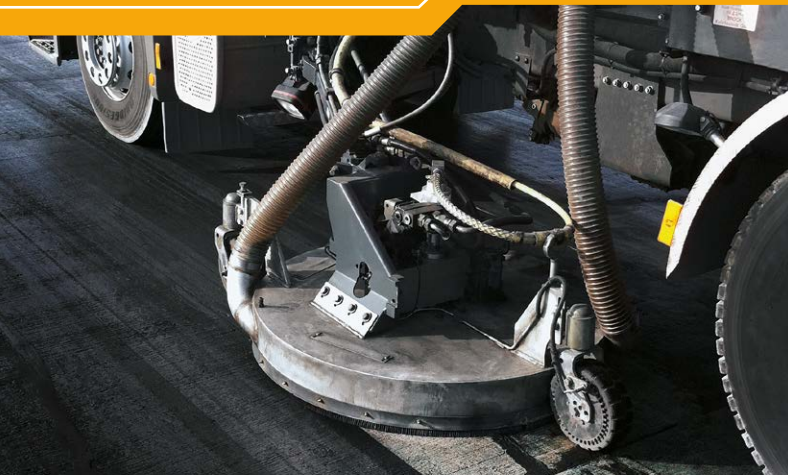
The surface cleaner in working position
