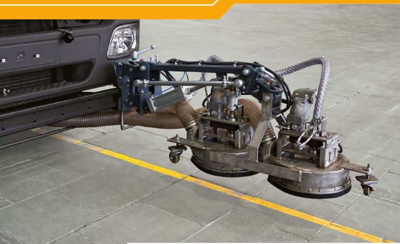
Removal device in front of the truck in lifted position
