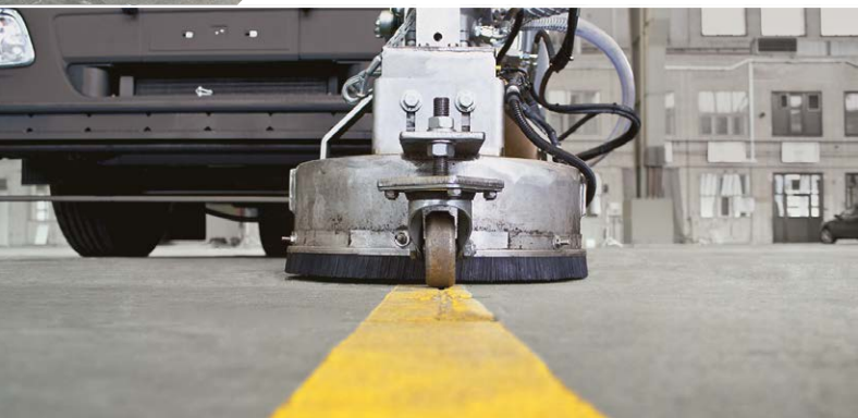
Height adjustable wheels keep the device in ideal working position
