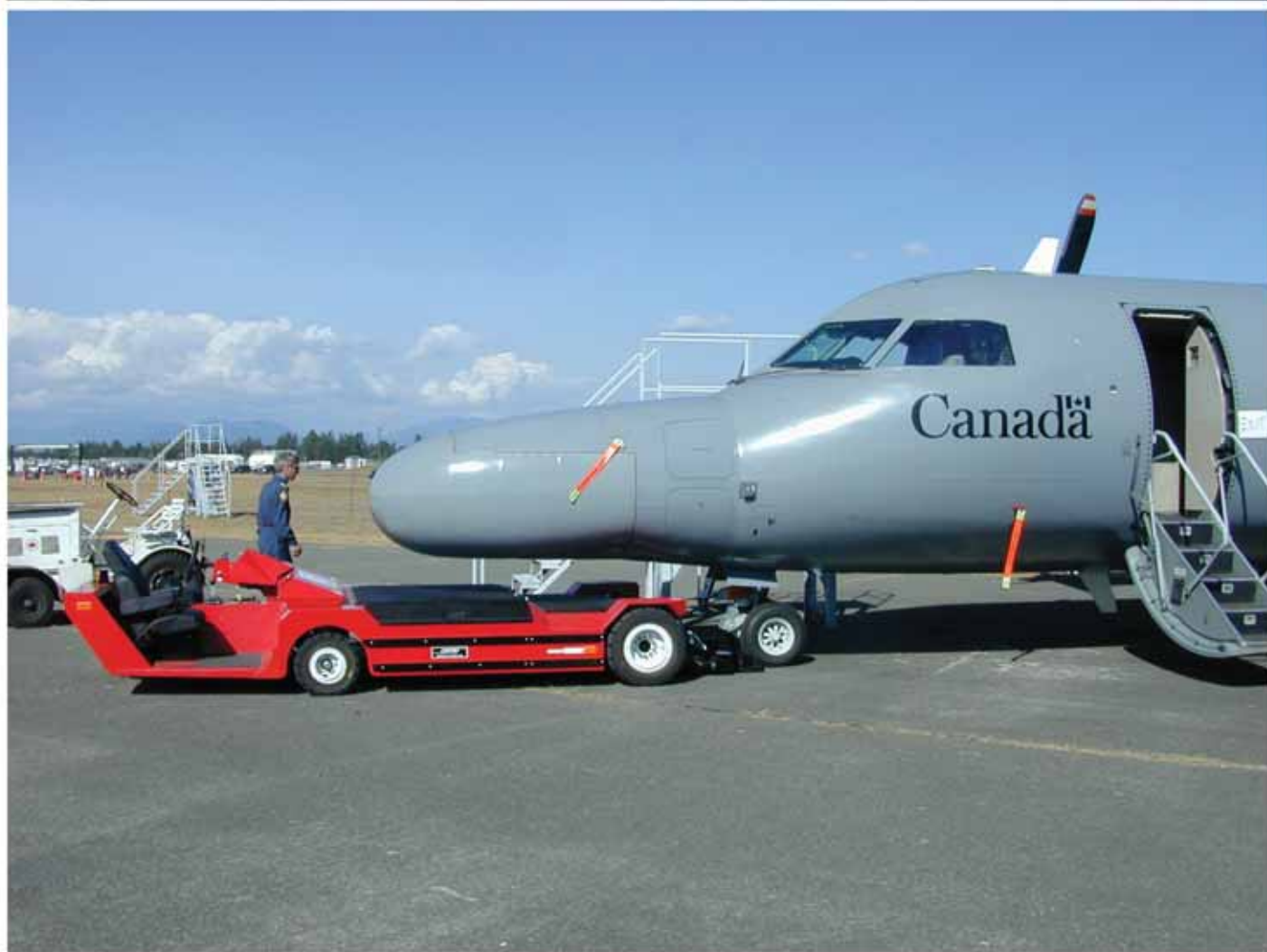
CFB COMOX / AIRSHOW 2001 / LEKTRO AP8850SDA TOWBARLESS AIRCRAFT TOW VEHICLE ON DEMO
