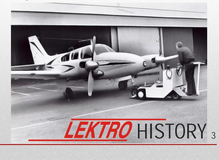
• Towbarless towing has been used by commercial airlines worldwide since the mid-1980s
