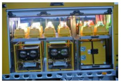
S4GA Trailer offered for the airport in Thailand contains a complete set of airfield lights to illuminate temporary runway within 20 min in accordance with ICAO regulations. It includes:
