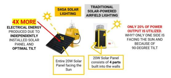
Some manufacturers of the traditional solar-powered lighting mount solar arrays into walls of the light casing. Although this solution works fine for temporary applications – in case of fixed (permanent) systems this kind of design has two significant disadvantages:
