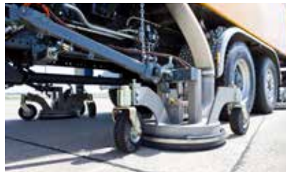
Both demarking devices in working position. Each device (3 x at the rear and 2 x at both sides) can be activated separately or in combination - the system is able to work on several and different applications.
