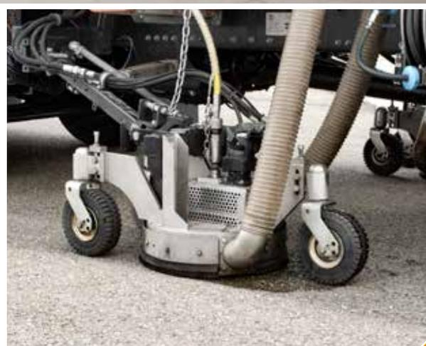
The ARC 3400<sup>®</sup> can be used professionally for roughening of road surfaces, rubber and paint marking removal as well as road and runway cleaning.
