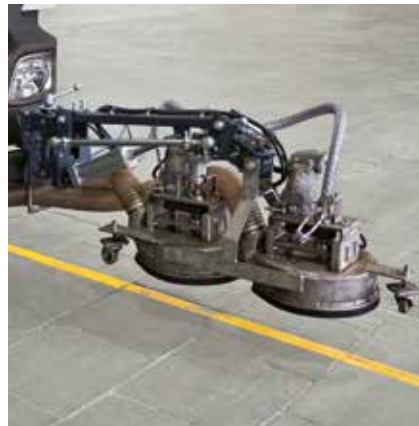
Removal device in front of the truck in lifted position
