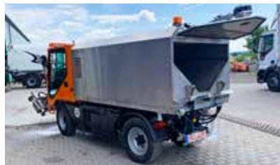
When the tailgate is opened the waste water tank can be cleaned easily.
